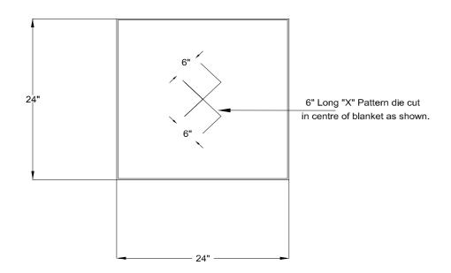
For field installation on the back of steel "lay-in" diffusers, or tappered neck diffusers in ceiling applications.
